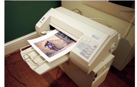
Introduced in late 1994, the Epson Stylus Color 720 dpi printer was, historically, the first desktop inkjet printer capable of producing "photo quality" prints.
